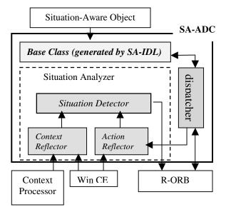
Figure 3: SA-ADC Architecture.
