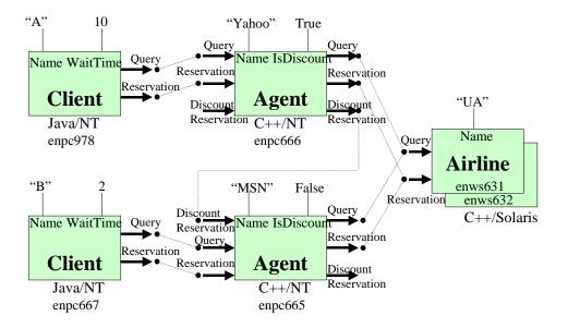
Figure 5: The component architecture of a simple Airline Reservation System
