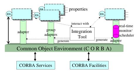
Figure 4: The role of the integration tool in constructing distributed component-based software
