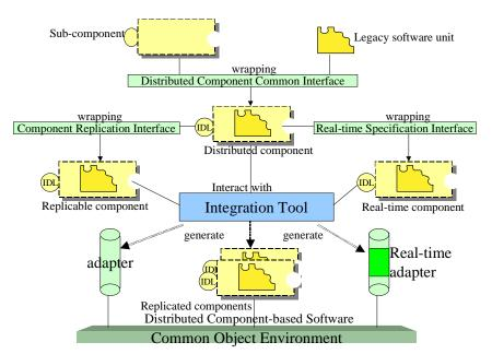
Figure 3: Our integration process of distributed components
